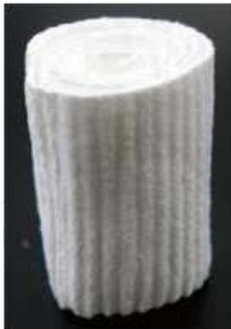
Fig. 8. Unidirectional porous HAp/Col bone-like nanocomposite.
