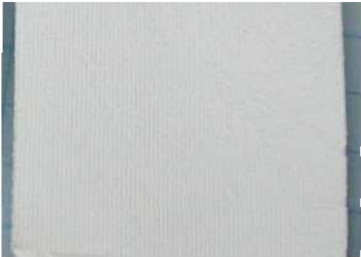
Fig. 6. Wavy membrane prepared from HAp/Col flexible membrane.
