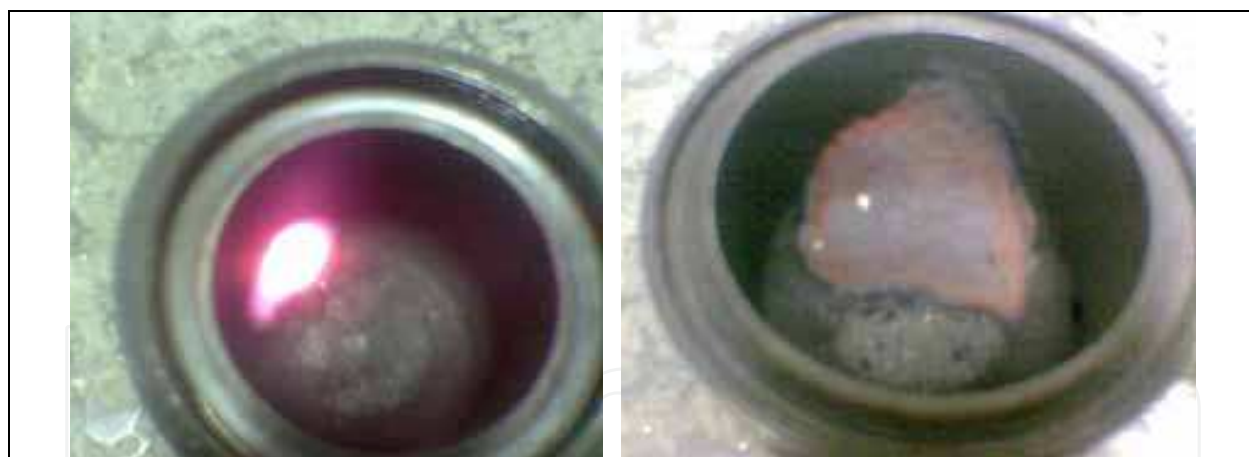
Fig. 14. Images of opened vial during combustion reaction of 3\text{Fe}_2\text{O}_3+8\text{Al} powder mixture.
