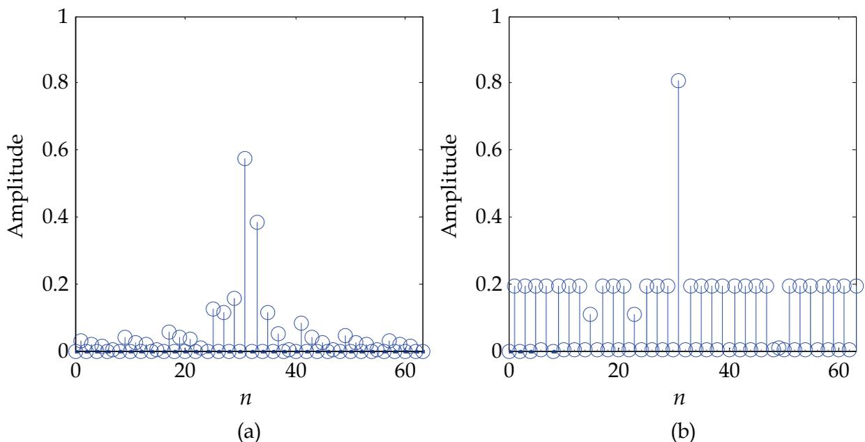
Fig. 4. Approximations to a discrete-time impulse using only inactive users. (a) Minimizing  $\ell_2$  norm. (b) Minimizing  $\ell_\infty$  norm
