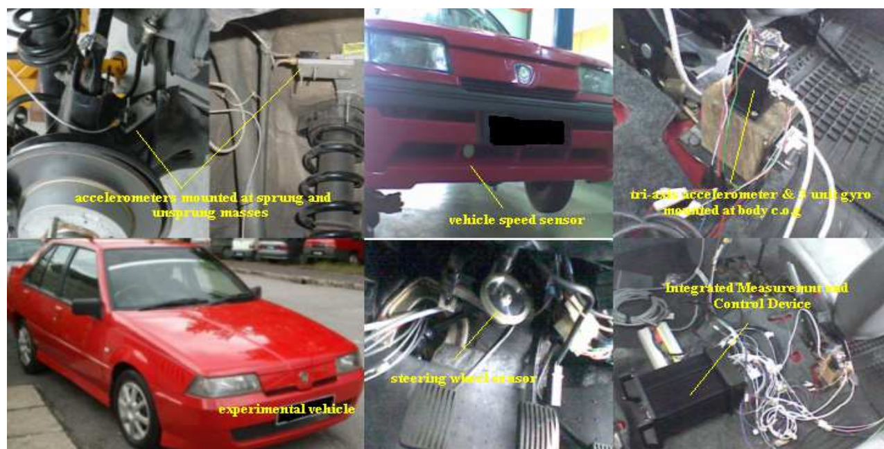
Fig. 5. Instrumented experimental vehicle
