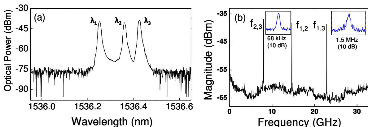
Fig. 2.22. (a) Optical spectra of lightwaves and (b) electrical spectra of their beat notes, where  $f_{1,2}$ ,  $f_{2,3}$  and  $f_{1,3}$  denote the beat notes generated by the lightwaves  $\lambda_1$  and  $\lambda_2$ ,  $\lambda_2$  and  $\lambda_3$ , and  $\lambda_1$  and  $\lambda_3$  respectively
