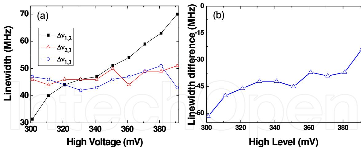
Fig. 2.20. (a) Linewidth measurement when fixing  $V_L$  at 300 mV and tuning  $V_H$  from 301 mV to 391 mV, and (b) Linewidths difference:  $\Delta v_{1,2} - (\Delta v_{2,3} + \Delta v_{1,3})$ , where  $\Delta v_{1,2}$ ,  $\Delta v_{2,3}$ , and  $\Delta v_{1,3}$  are 6-dB linewidths of beat notes between  $\lambda_1$  and  $\lambda_2$ ,  $\lambda_2$  and  $\lambda_3$ , and  $\lambda_1$  and  $\lambda_3$ , respectively
