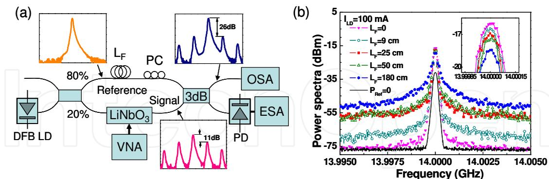
Fig. 2.2. Investigation of interference between lightwaves from one laser source. (a) Experimental setup. PC, polarization controller;  $L_F$  is the fiber length difference between two arms of the M-Z interferometer. (b) Measured power spectra at various fiber length differences. The curve " $P_{ref}=0$ " indicates the spectrum without reference signal injection. The inset shows the higher resolution spectrum
