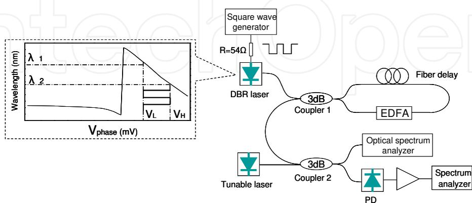
Fig. 2.21. Delayed optical self-injection system
