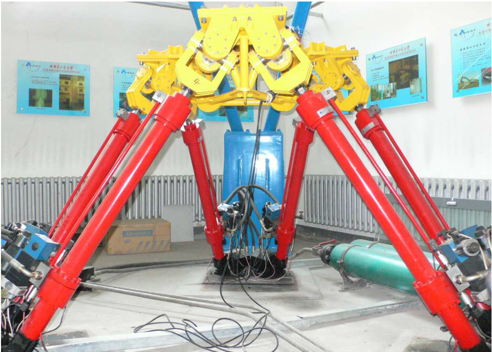
Fig. 4. Experimental hydraulic 6-DOF parallel manipulator
