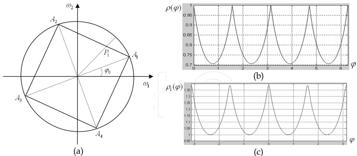
Fig. 10. (a) Square inscribed in the circle of radius  $R$  in the frequency plane, with an initial phase  $\varphi_0$ ; (b) periodic function  $\rho(\varphi)$ ; (c) its periodic approximation  $\rho_1(\varphi)$
