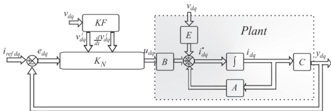
Fig. 13. Block diagram of the proposed LQR system.
