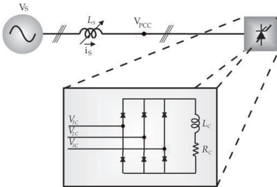
Fig. 3. Open loop system with variable line inductance
