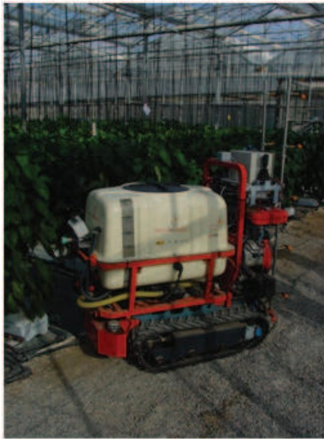
Fig. 17. Mobile robot for agricultural tasks
