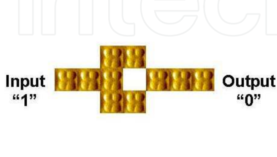
Fig. 5. Schematic display of QCA inverter changing data from “1” to “0” or from “0” to “1”
