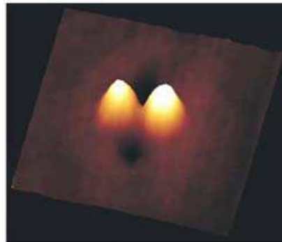
Fig 18. Bi-quantum dot molecule grown on quantum ring
