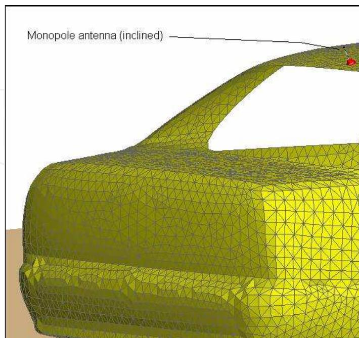
Fig. 6. Monopole antenna (inclined) mounted on a car
