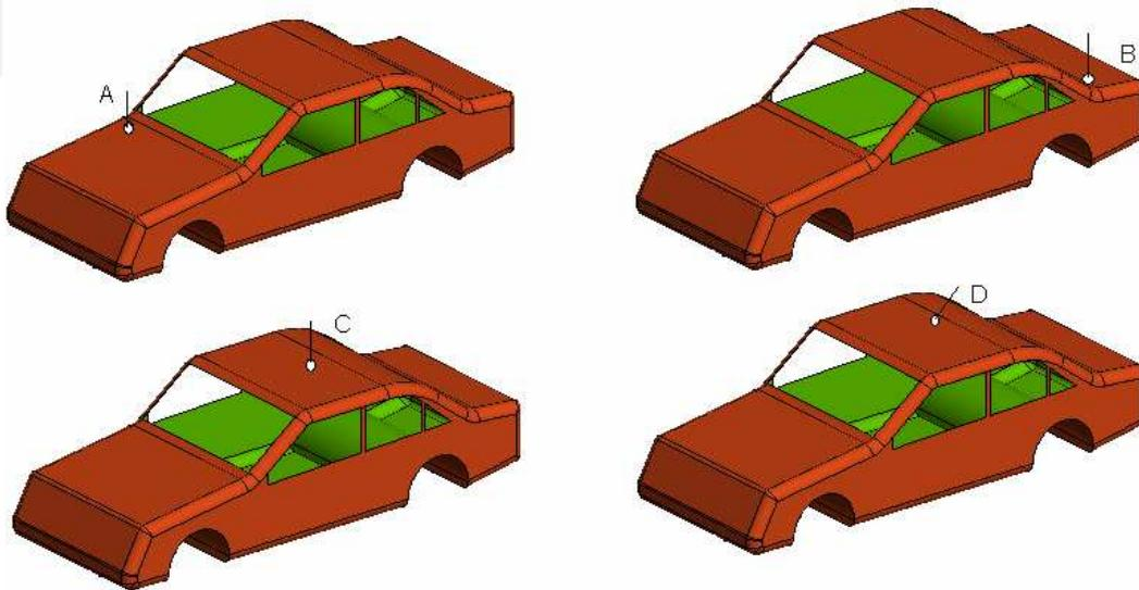
Fig. 7. Monopole antennas mounted at various locations
