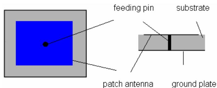
Fig. 10. Square/ rectangular patch antenna
