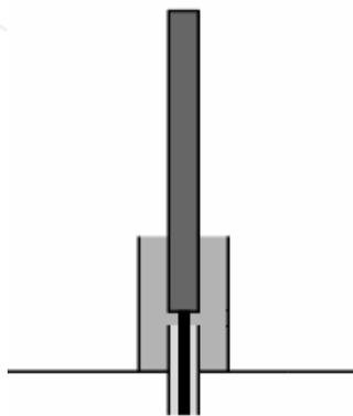
Fig. 4. Monopole antenna with sleeve
