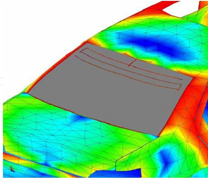
Fig. 16. Current distribution due to integrated windscreen antennas
