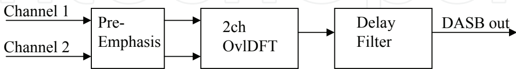
Fig. 14. FPGA design diagram of DASB
