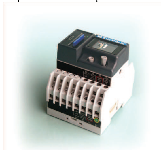
Fig. 4. Prototype of the three-phase, voltage-and-current, 61000-4-30 Class A power quality monitor. The digital camera influence can be seen in the SD memory card, which holds up to 2 000 MB of data. Standard DIN-rail mounting means installation is cheap and quick.
