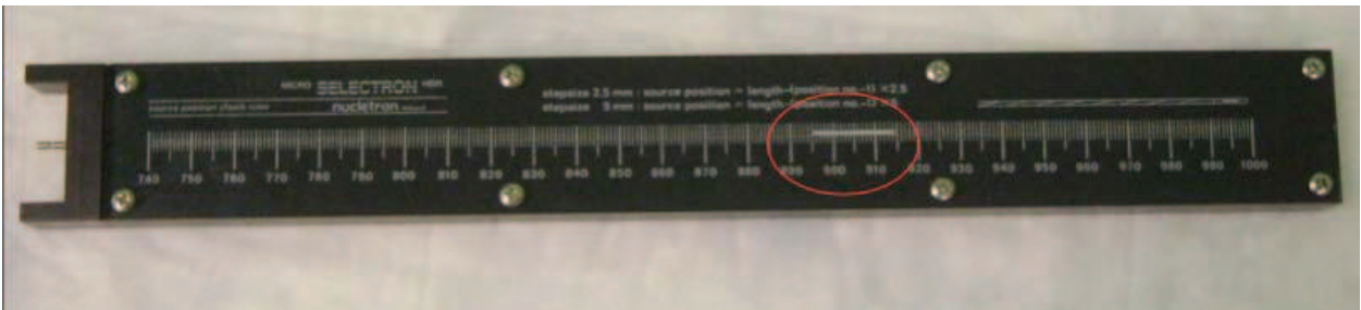
Fig. 6. The source position ruler showing the source in a red circle
