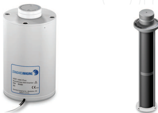
Fig. 5. A typical well-type ionization chamber, including a tool to perform tests of source positioning within 0.3 mm, timer accuracy, and consistency of source activity
