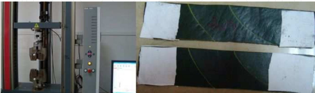
Fig. 10. The tension test of plant leaf
