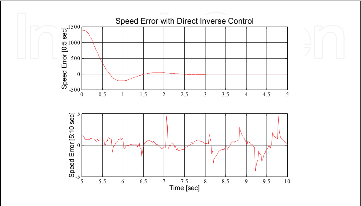
Fig. 12. Speed error due to a step reference signal
