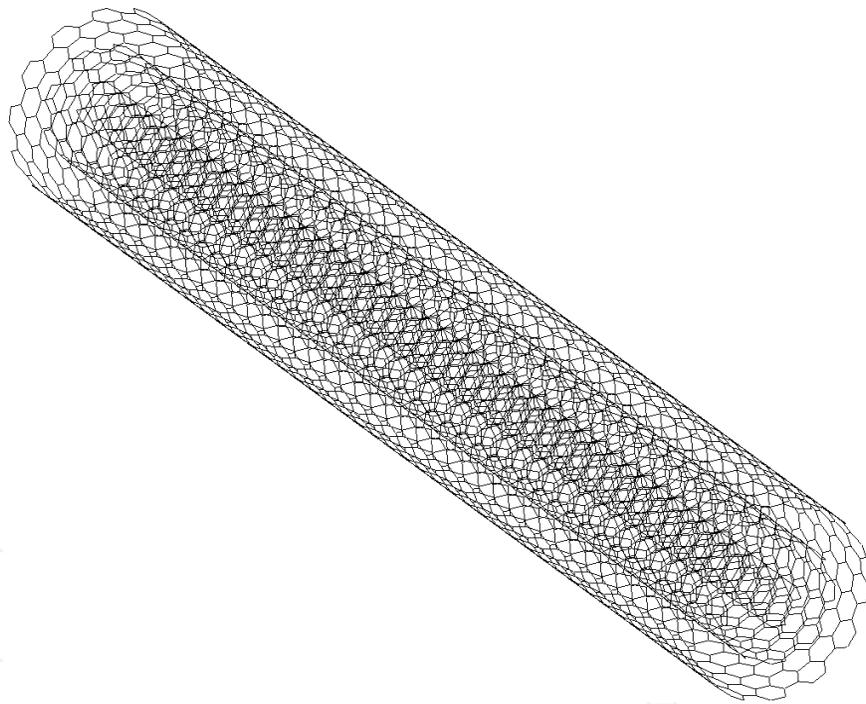
Fig. 3. Geometry of a multi-walled CNT.
