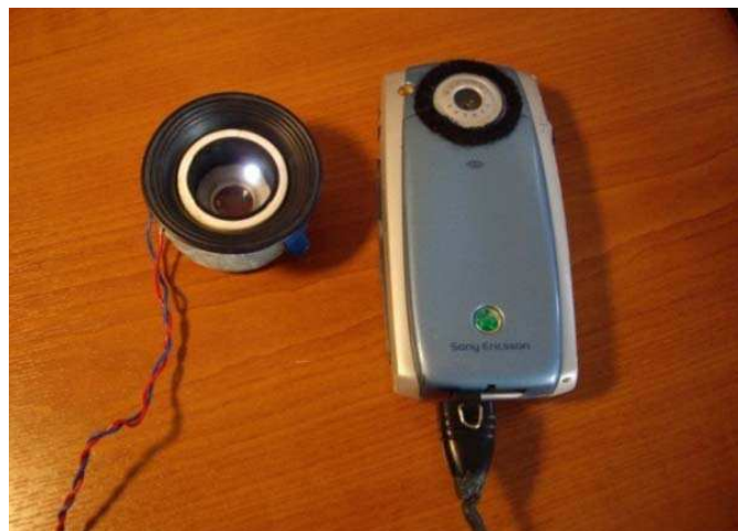
Fig. 6. An 'Eye Cup' with a Luminous Diode links to the Sony Ericsson P800 Mobile Phone
