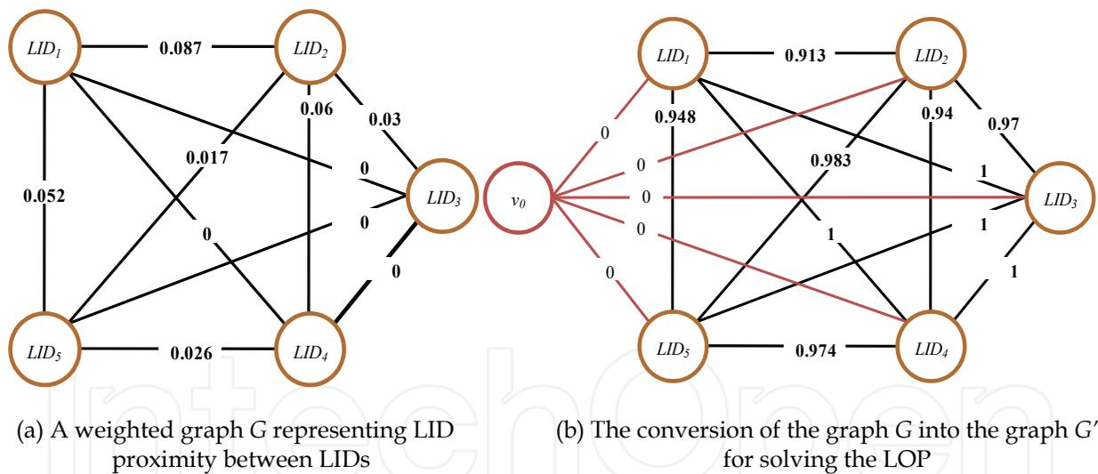
Fig. 5. An example of a weighted graph for reordering LIDs based on LID proximity
