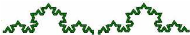
Fig. 5. Standard Koch fractal dipole antenna. Table 1 summarizes the standard Koch fractal dipole antenna properties with different fractal iterations at reference port of impedance 50\Omega . These dipoles are designed at resonant frequency of 900 MHz.
