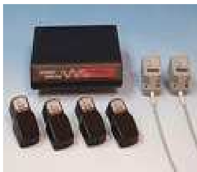
Fig. 3. Patriot wireless electromagnetic tracker
