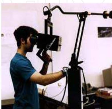
Fig. 2. A Binocular Omni-Orientation Monitor (BOOM)
