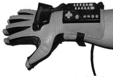
Fig. 5. An instrumented glove (Nintendo power glove)
