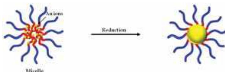
Fig. 1. Schematic illustration to prepare the surface modified Au NPs via (a) grafting from, (b) grafting to, (c) ligand exchange and (d) templating methods.
