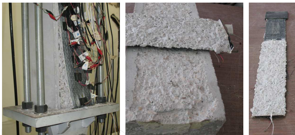
Fig. 11. Specimen after test and typical failure mode
