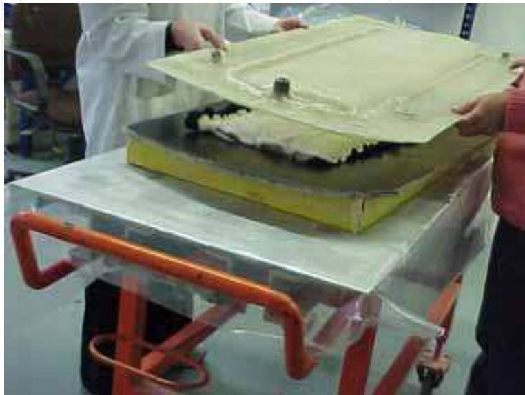
Fig. 42. Exterior mould – inferior and superior components
