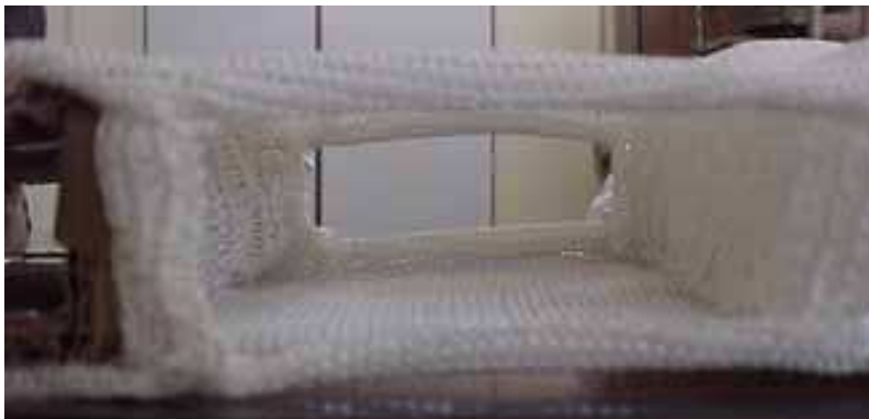
Fig. 24. Sandwich fabric with connecting knitted layers
