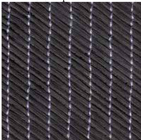
Multi-axial fabric made of carbon fibre
