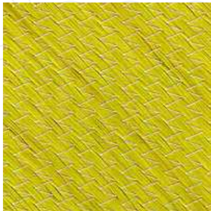
Multi-axial fabric made of Kevlar fibre
