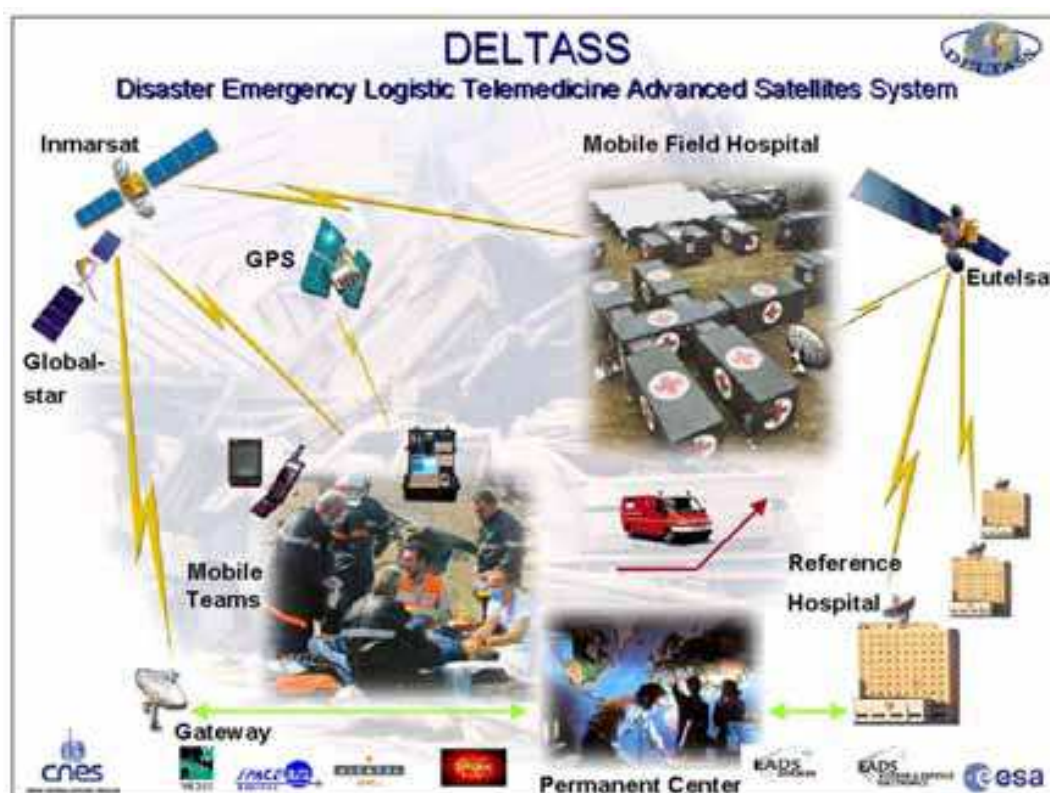
Fig. 2. DELTASS System Architecture: Mobile Teams, Permanent Center (PC), Mobile Field Hospital (MFH) and Reference Hospital (RH) are interconnected via several satellite systems with different bandwidths. Additionally terrestrial communication channels support the data exchange between the PC and the RH.
