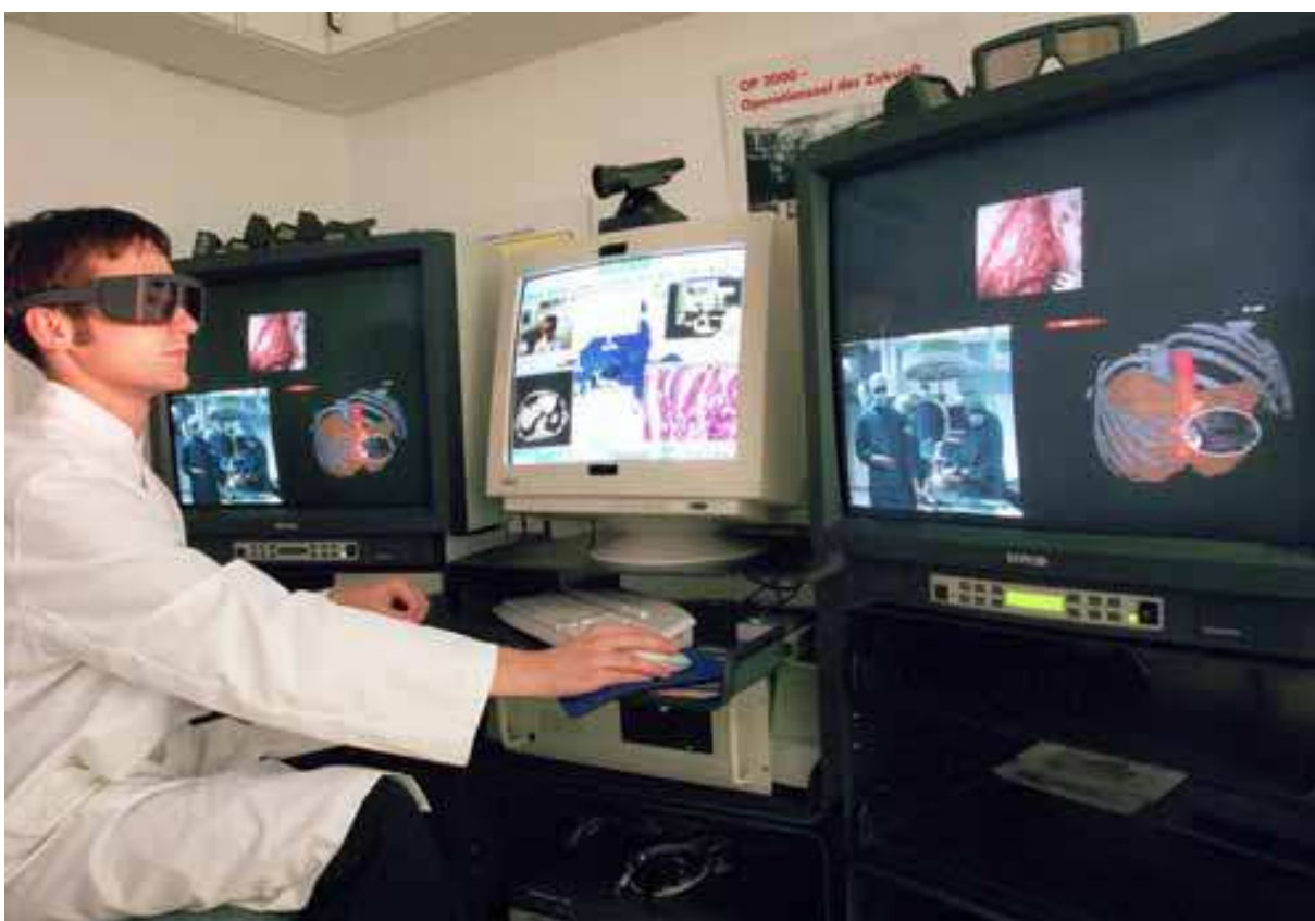
Fig. 13. Workplace 2020 for Surgical Oncology: Stereoscopic visualisation and real-time interactive video communication
