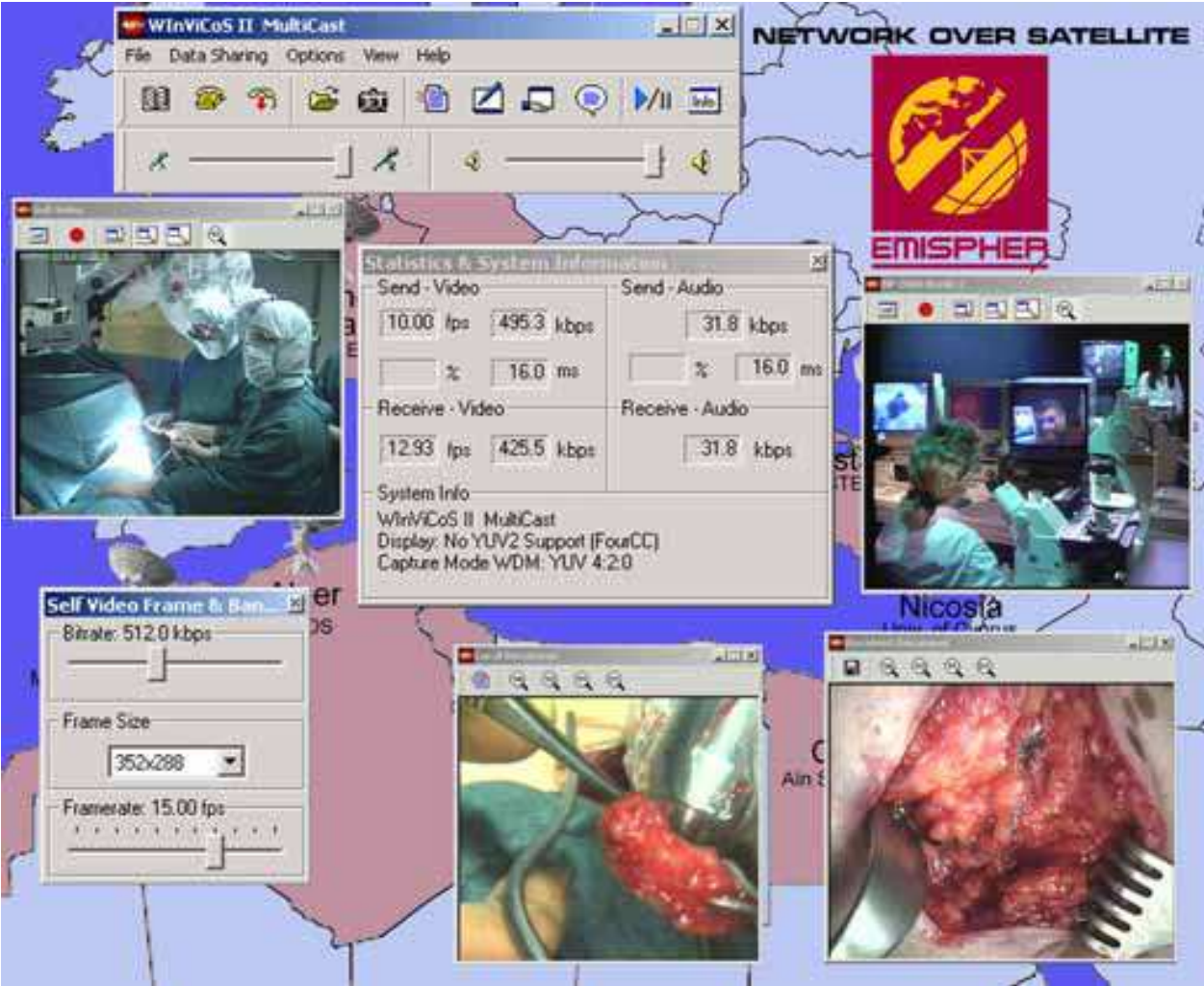
Fig. 1. WinVicos main user interface (top): two live video windows (top) and two still-image windows (bottom), online flexible adjustment of transmission parameters (bottom left), transmission performance can be monitored online (center). In both the video windows and the still-image windows WinVicos supports the use of common cursors shared by the conference partners. As WinVicos is an all-software system
