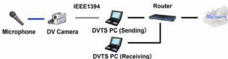
Fig. 2. Minimal configuration for DVTS setup
