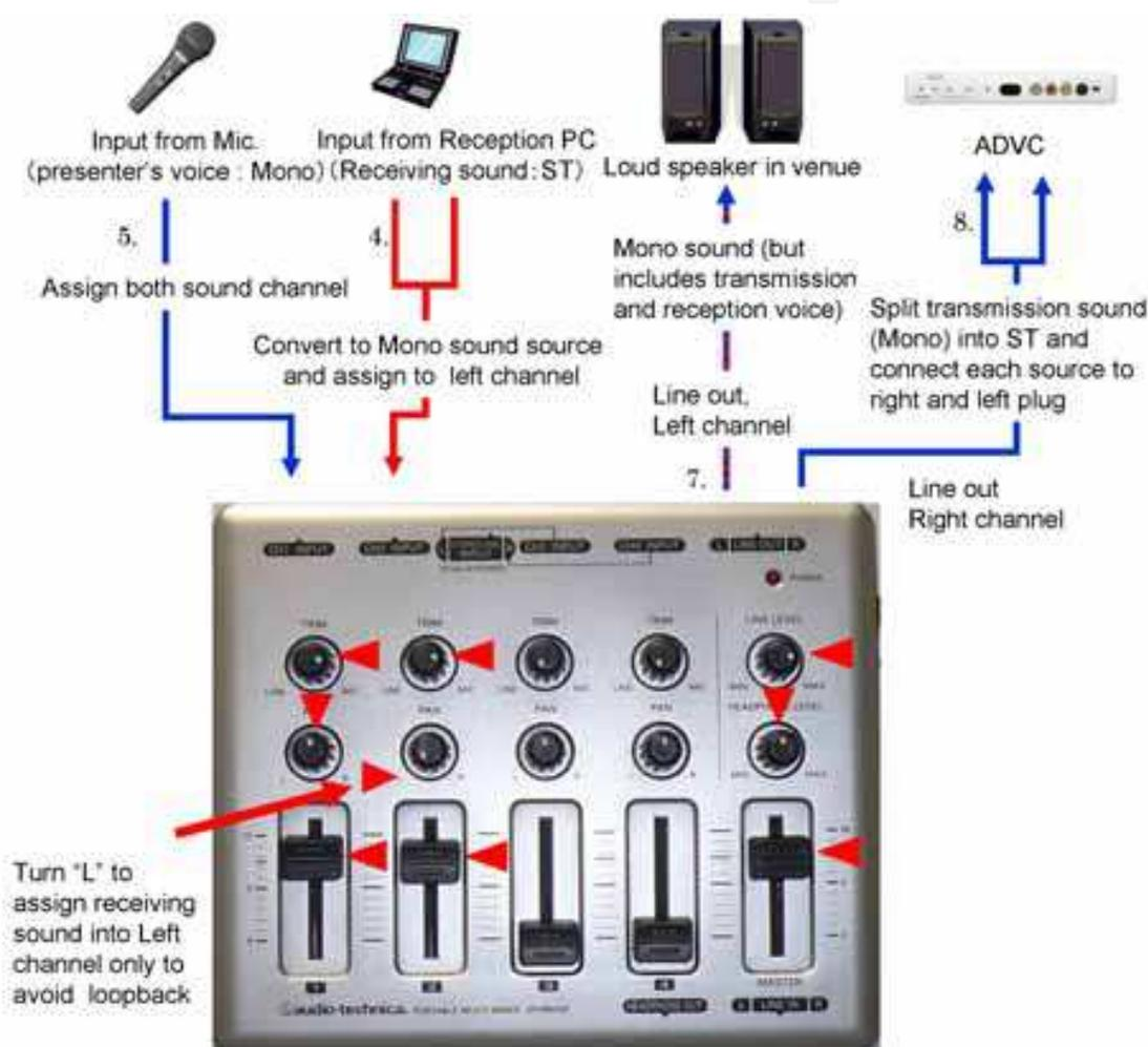
Fig. 4. Configuration diagram for setting audio
