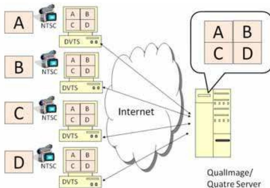
Fig. 5. Mechanism provided by QualImage/ Quatre system
