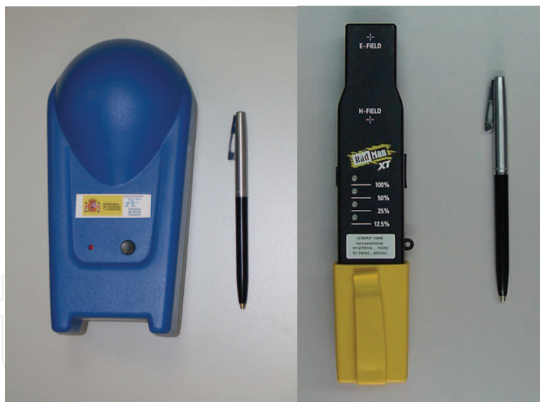
Fig. 1. Antennessa EME SPY and RadMan XT dosimeters
