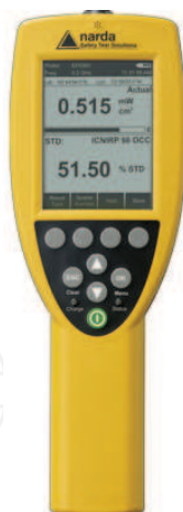
Fig. 5. Narda Broadband Field Meter NBM-550
