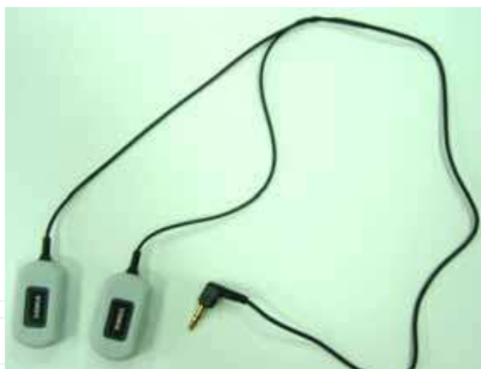
Fig. 16. Developed bone conduction vibrator speaker
