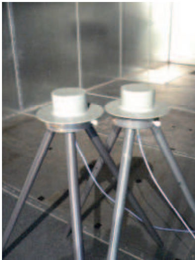
Fig. 3. The interior of the reverberation chamber with two conical monopole antennas
