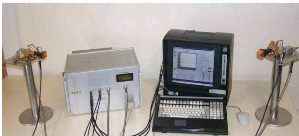
Fig. 1. Channel sounder at 60 GHz realized by IETR
