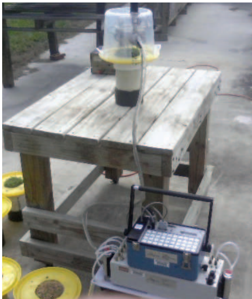
Fig. 9. Portable chamber system for measuring canopy gas exchange
