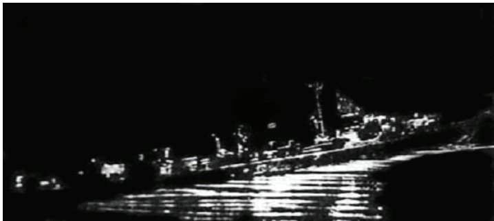
Fig. 3. The optical simulation results of electromagnetic waves scattering by the ship
