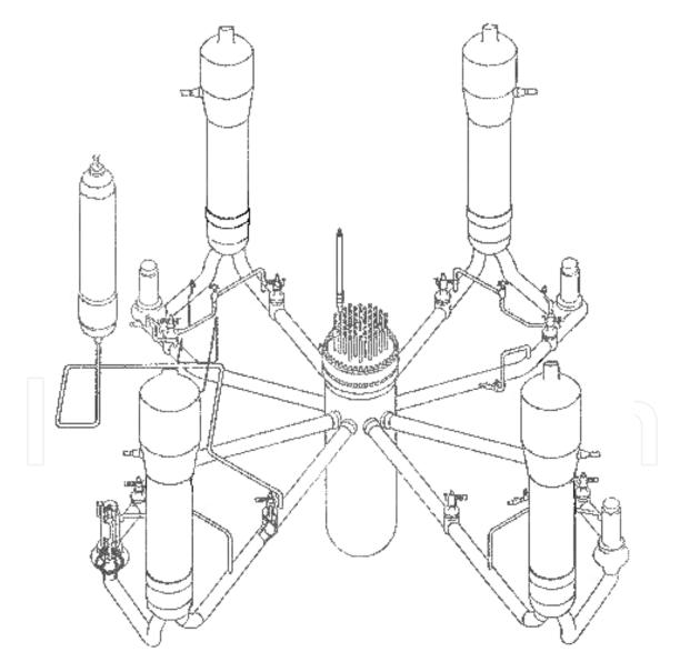
Fig. 2. General scheme of PWR primary circuit
