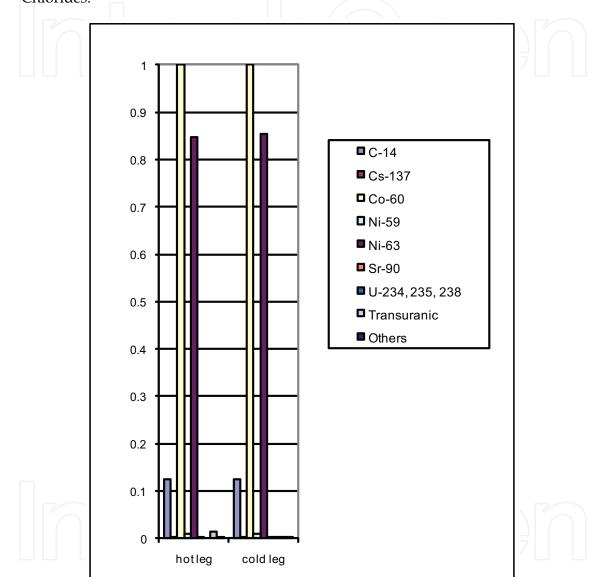
Fig. 5. Example of isotopic composition of contamination inside one of the steam generators of a decommissioned NPP
