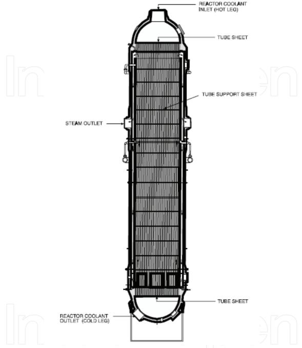
Fig. 3c. Typical Babcock & Wilcox Once through steam generator
