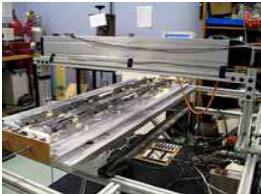
Fig. 51. Morphing wing system in the bench test
