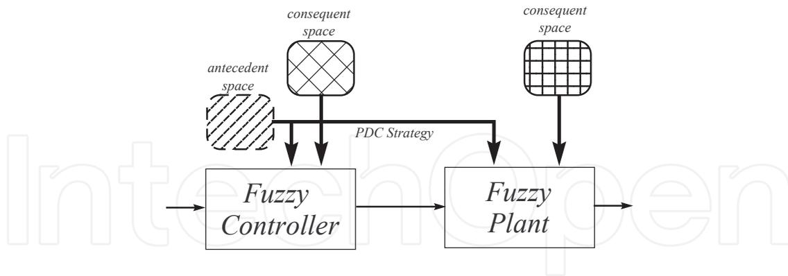
Fig. 4. Controller and plant fuzzy model in open-loop share the same fuzzy sets in the antecedent space.
