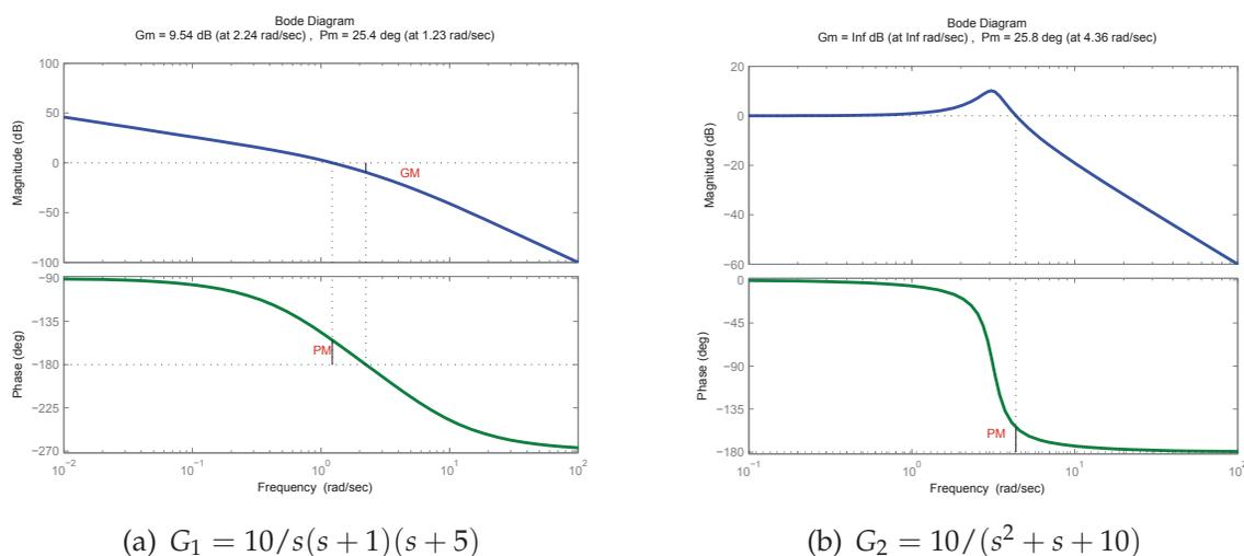
Fig. 2. The phase (9.54dB) and gain (25.4dB) margins of the system  $10/s(s+1)(s+5)$  is showed in (a). The phase (25.8dB) and gain (inf.) margins of the system  $10/(s^2 + s + 10)$  is showed in (b). Note that the gain margin of a first or second-order system is infinite since the polar plots for such systems do not cross the negative real axis.
