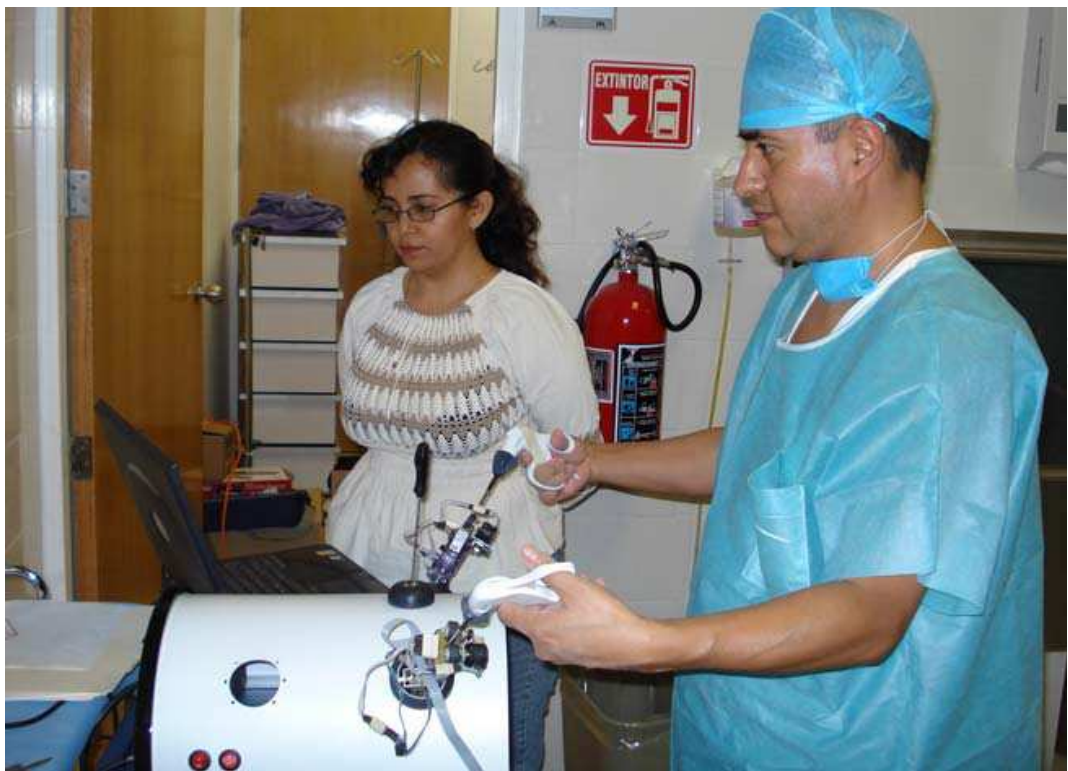
Fig. 4. General set up of the instrumented trocar installed in the trainer. The image shows the arrangement during the training.
