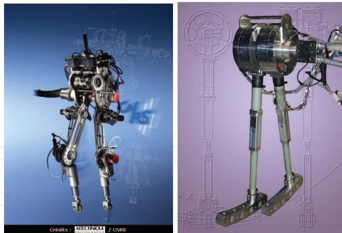
Fig. 1. Biped bipeds, “Rabbit” (left) and “Emu” (right).
