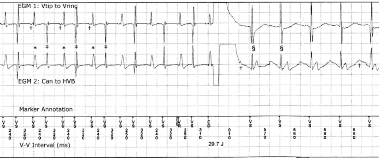
Fig. 5b. Inappropriate shock delivery caused by double counting. Intrinsic rhythm: sinus-arrest, considerable prolonged AV-conduction time (560 ms). * = intrinsic QRS-complex. PM rhythm: atrial pace-ventricular pace: † = paced p-Waves, ‡ = ventricular pacing artifact, prior to the shock ineffective due to pacing in the intrinsic ventricular refractory period. § = after shock delivery (CD) effective AV-sequential ventricular pacing by the PM, sensed by the ICD.
