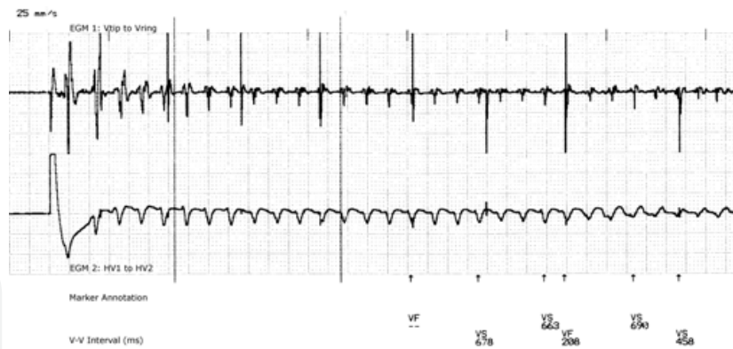
Fig. 26. Undersensing of a VT (induced by T-wave-shock) after reduction of ICD-sensitivity (Ventak Prizm 2VR 1860; Guidant) as reaction to overcounting of PM artifacts (Kappa KDR 401; Medtronic, bipolar leads!). The PM artifacts can be seen in the ventricular pace-sense-channel (top) as well as in the ventricular EGM of the defibrillation coils (bottom) and are being detected inconsistently by the ICD.
