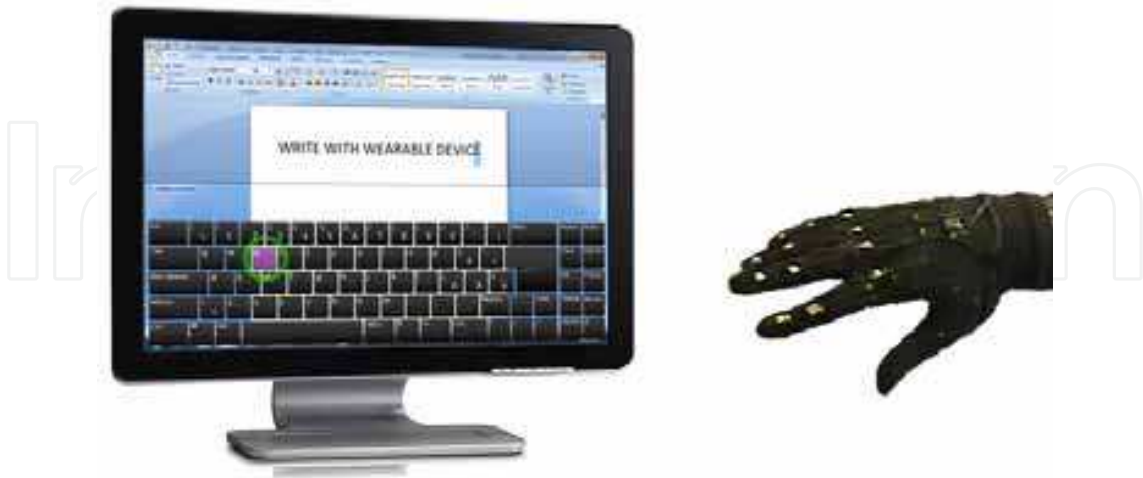
Fig. 4. Mouse and keyboard are unnecessary if computer interactions are made by a sensorized glove capable to accept commands obtained by finger motions.
