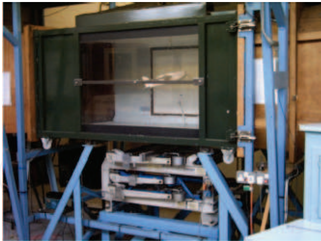
Fig. 1. The flexible suspension system for wind tunnel
