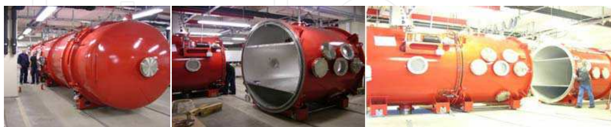
Fig. 4. Photographs of the (10m long) AWTS-II facility showing the mobile environmental chamber sections, the central test section can be removed laterally.
