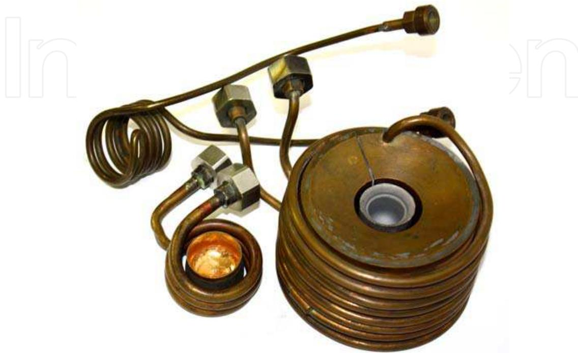
Fig. 2. Photographs of water-cooled evaporating inductors for use in electronics, two of them are shown with crucibles. The left inductor has the top turn with opposite winding as compared with the rest turns
