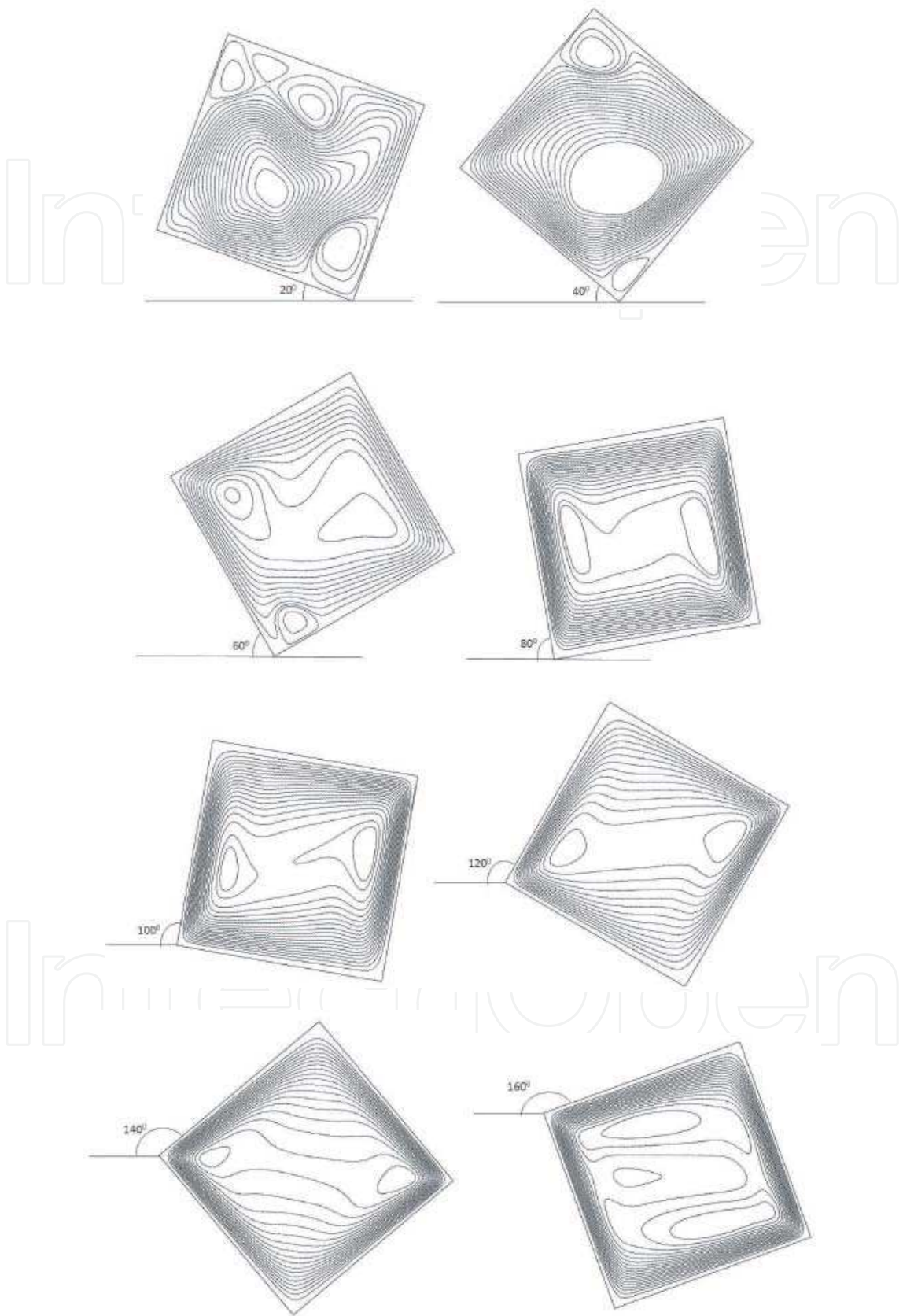
Fig. 6. Streamlines plots at Ra = 10^6 .
