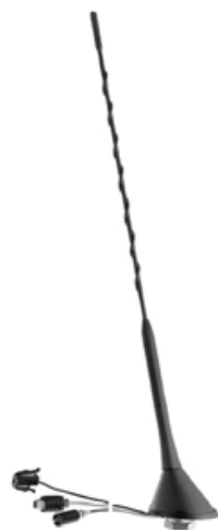
Fig. 6. Bee sting antenna © IEEE with permission (Cerretelli & Biffi Gentili, 2007)
