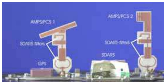
Fig. 10. Internals of a modern shark-fin antenna © IEEE with permission (J.F. Hopf et al., 2007)
