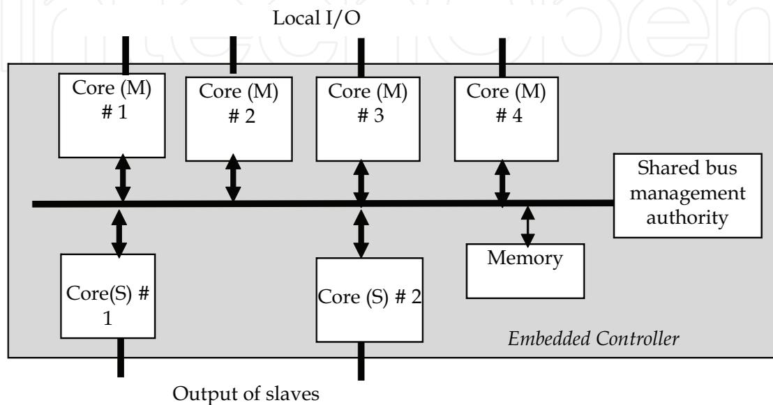
Fig. 2. Shared bus Integrated Multicore Embedded Controller
