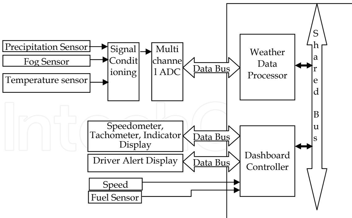
Fig. 12. Embedded controller for driver alert message display
