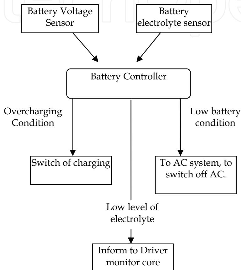
Fig. 10. Flow diagram of working of battery controller
