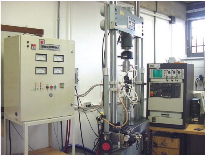
Fig. 6. Overall view of the testing apparatus, showing the induction furnace and the MTS 810 servo-hydraulic testing system.
