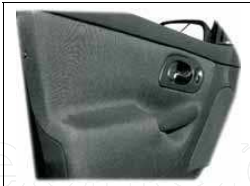
Fig. 2. Example of an integral door panel
