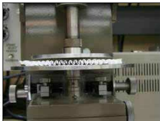
Fig. 20. Customization of the KES-FB3 compression tester
