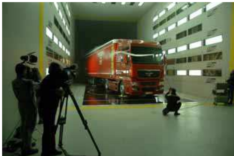
Fig. 7. Truck in 9.5x9.5 test section
