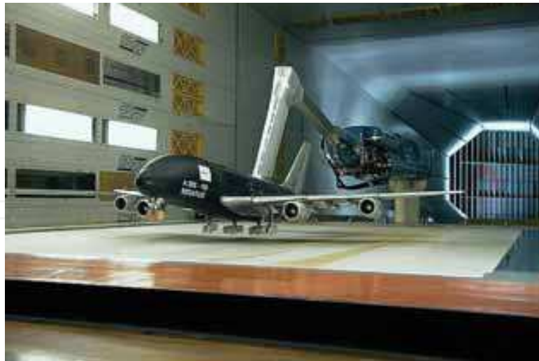
Fig. 6. Model on sting above moving belt
