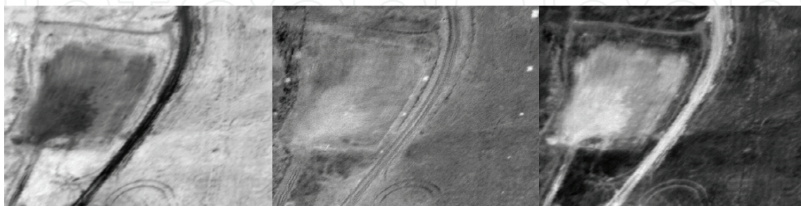
Fig. 10. Three frames of a movie sequence showing the differences from average for band indices 6, 34 and 52. The targets are invisible in bands 6 and 52 but visible in band 34. In this case we also applied dynamic noise reduction in which the temporal noise is reduced (see text). This latter transformation is not strictly necessary since the human visual system is highly robust to noise.
