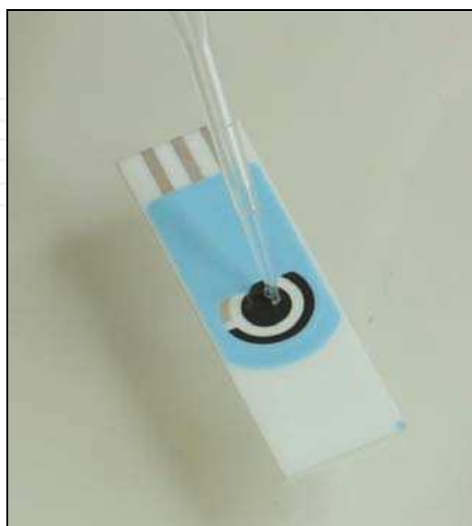
Fig. 8. Screen printed electrode used for biomediator immobilization.
